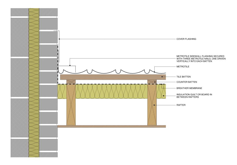
Metrotile Abutment Detail With Sidewall Flashing
