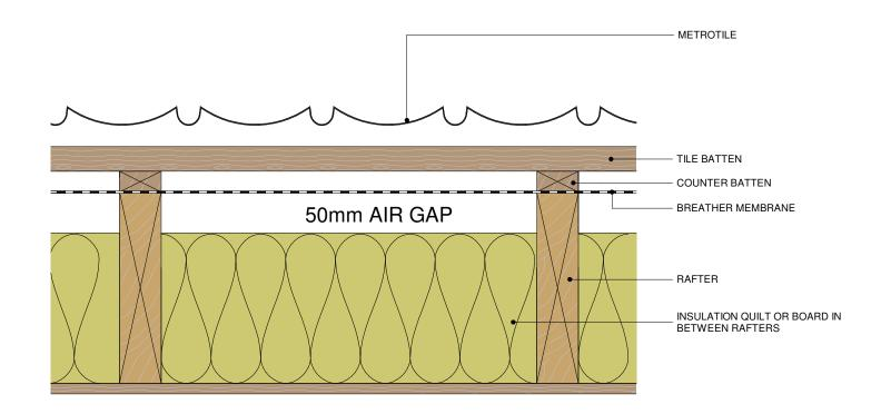
Metrotile Longitudinal Section Detail
