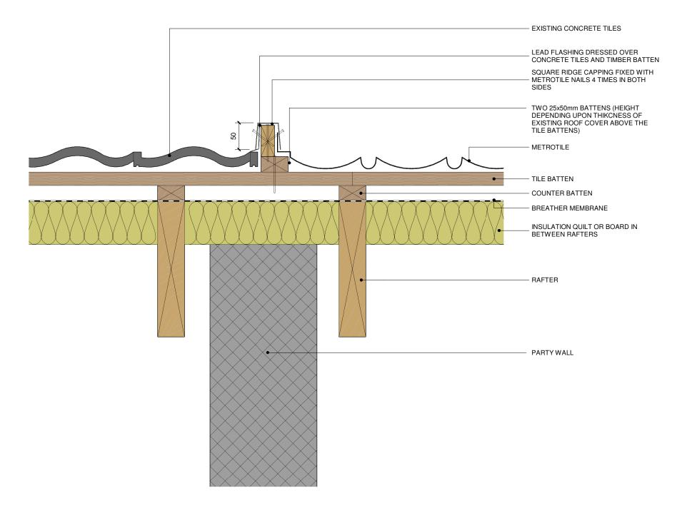
**Metrotile Step Detail Abutting Concrete Tiles**
