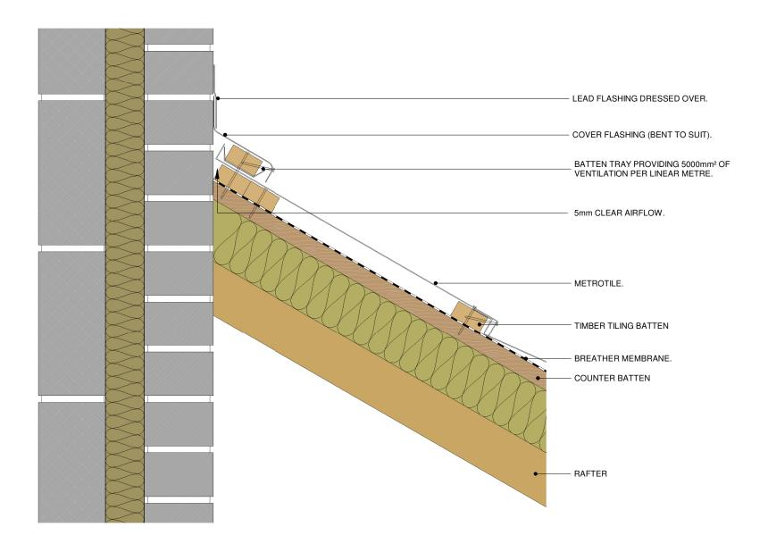
Metrotile Abutment Ridge Ventilation Detail
